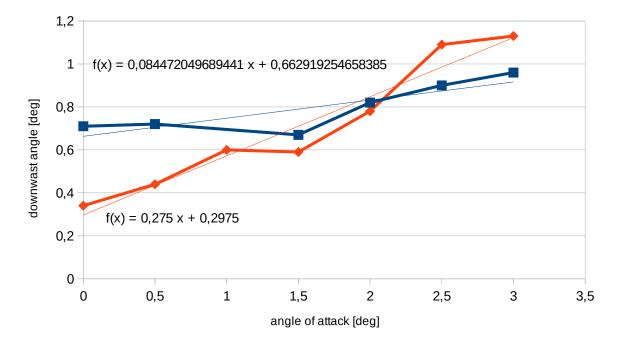
At Y= 0,5 m change is 0,08447 deg/deg at Y= 1,0 m change is 0,275 deg/deg
