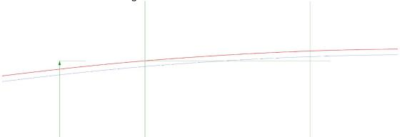
Width of spar box can be variable. Width is interpolated between these three Y locations. In Pik28 spar has constant width, for simpler manufacturing. A width of 100 mm is because that is the common tape width for carbon and glass unidirectional reinforcement.
