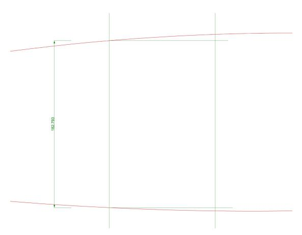
First determine which corner is the slimmest. In picture above at top the front side of box is lower and also at bottom the front side is upper. It can be otherwise if profile is cambered. For calculation a square sparbox is used.
