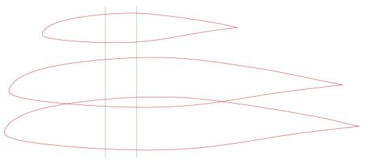
Easily visible is that the thickest part of this 15% thick profile is aft of the spar box. This picture uses same width for spar box in every location. It can be variable, then intermediate locations are interpolated. The meaning of thickness at spar location (ref #1) is illustrated below. You have to measure distances and convert them to % (of c) values, because calculations uses this. In this location chord length is 1305,8 mm.
