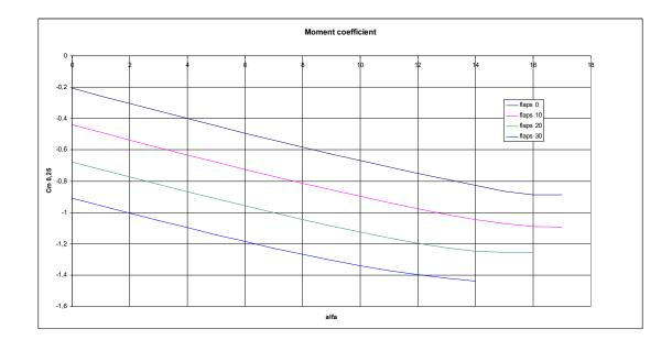
ASTM 5.2.2.4 states to use moment coefficient of at least +/- 0,025, the calculated values are more, so they are used.
