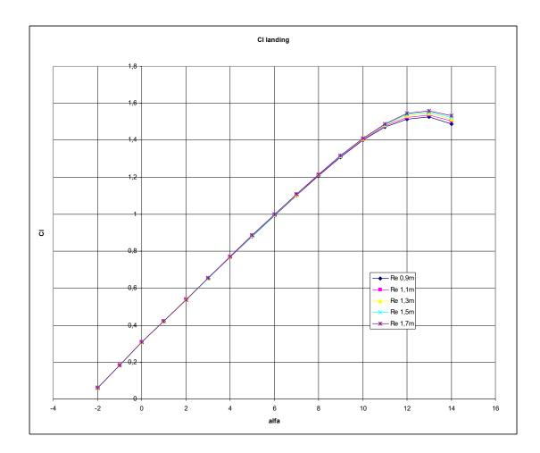
For flap deflection no wind tunnel data was available. Airfoil characteristics were estimated using calculation programs.
