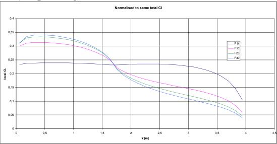
Lift curves for wing was calculated using wing-loading of 560,7 N/m<sup>2</sup>. This represents flying weight of 499 kg. Difference (in distribution) in results is negligible for other weights.
