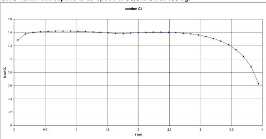
Graph for alfa 16 deg with flaps at 0 deg corresponding to Wing Cl of 1,475 which correspond to air speed of 93,8 km/h at 499 kg.
