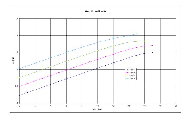
Maximum lift coefficients and corresponding stall speeds @499 kg. Stall speed at forward c.g.:
