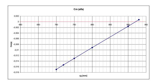
This yields neutral point of 922 mm (45,2% MAC). Which is in close proximity of analytical results (above). Analytical result for neutral point is 5% aft of the stick free neutral point value.
