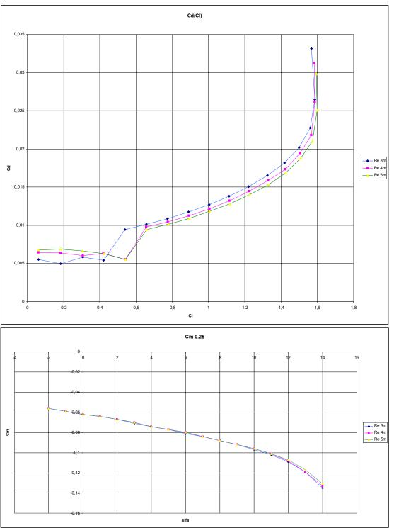
Laminar flow dip ends at about Cl 0,6, which represents air speed of 140 km/h @ 499 kg or 153 km/h @600 kg. So it is safe to say at at cruise speed aircraft wing is working in low drag angle of attack.
